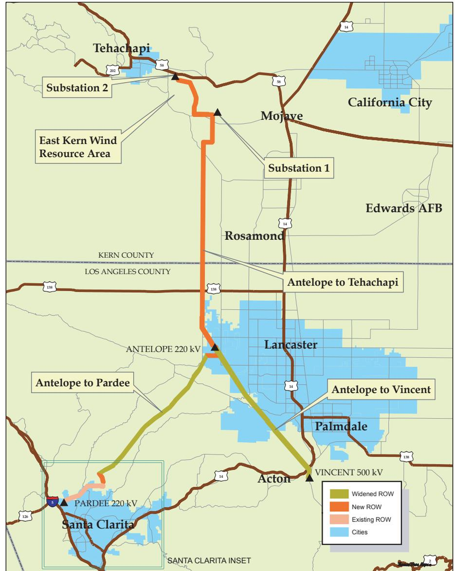
a combination of new and existing rights of way. The first 1.1 miles of line from Antelope Substation would be constructed within a new, 180 foot-wide right-of-way. From that point, and for the next 17.5 miles, the new 500 kV transmission line would replace a 66 kV line within an existing SCE right-of-way. The width of the first 4.6 miles of existing SCE right-of-way would need to be increased to 180 feet. At mile
